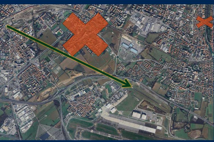
Arrival from the North: expect to join left downwind or base at 1500 ft. Caution to avoid P area north of the airfield and noise sensitive area on final. (do not turn on base until abeam Bergamo train station)
