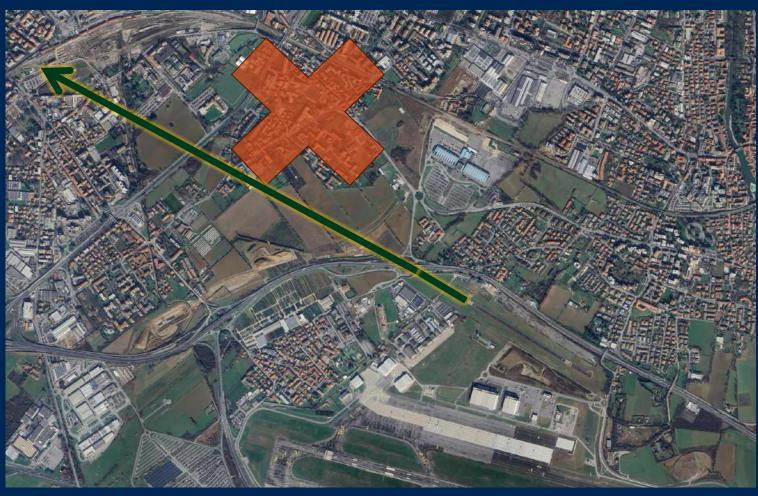
Departure to the North: after takeoff fly track 295°, do not turn right before reaching 1500 ft and not before Bergamo train station, due to noise sensitive and P areas, then continue as cleared.
